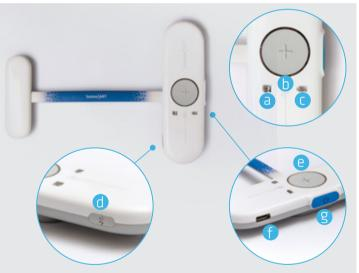
(a) Memory LED(b) Recording LED(c) Battery LED
